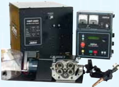
Hot Wire GTAW/PAW Process
